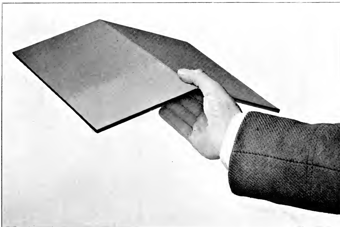
FIG 72. ALLEGED FAULTY BESSEMER PLATE, 1875
