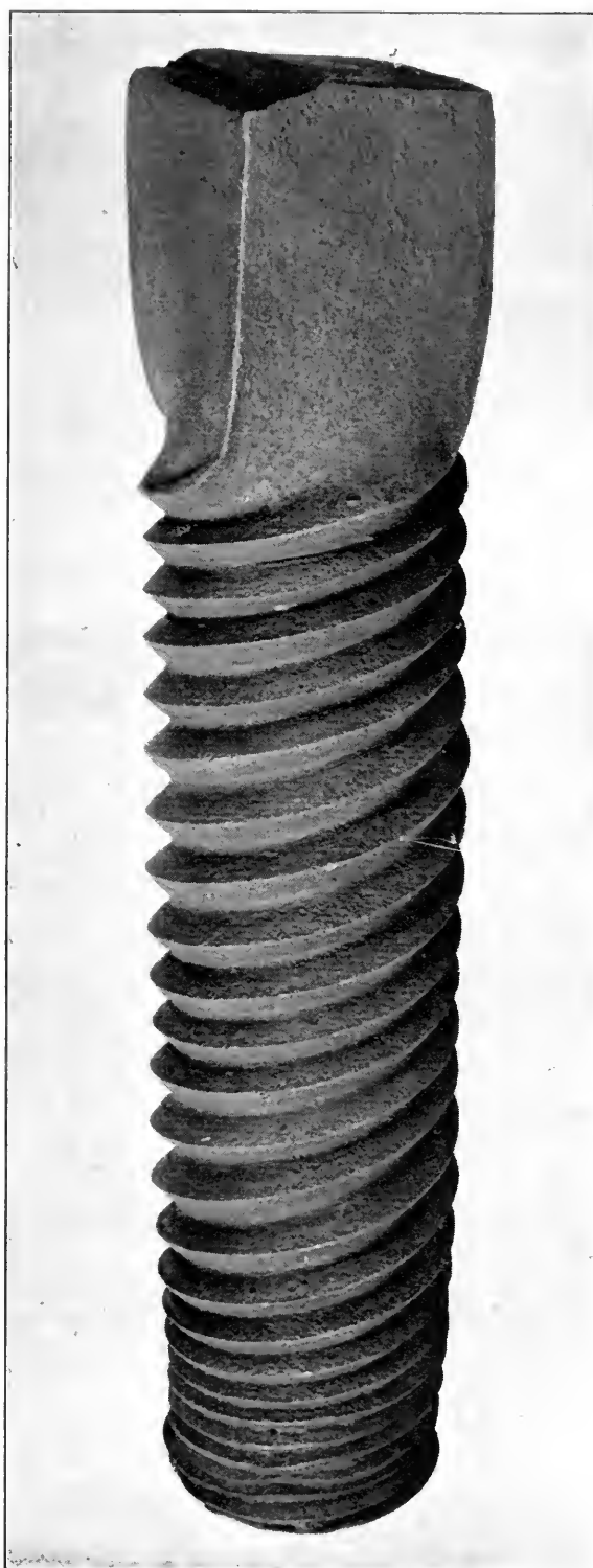
FIG. 58. SQUARE BAR OF BESSEMER STEEL TWISTED COLD, AND SHOWN AT SHEFFIELD, 1861
